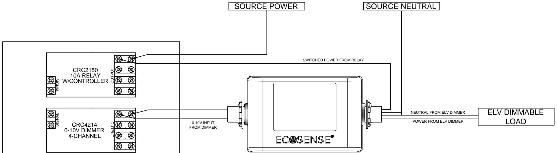
**NOTE:** IF FLICKERING OCCURS; ADJUST THE "LO" TRIM LEVEL ON THE CRC4214 CLOCKWISE UNTIL THE LOAD OUTPUT BECOMES STABLE. THE ADJUSTMENT SHOULD BE AS MINIMAL AS POSSIBLE TO RETAIN BOTH A STEADY LIGHT OUTPUT AND PRESERVE MAXIMUM DIMMING RANGE.
